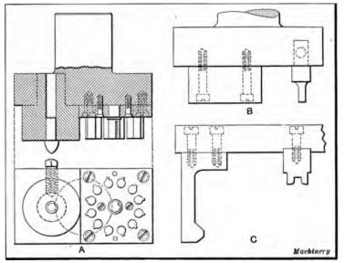
Fig. 21. Different Types of Punches
